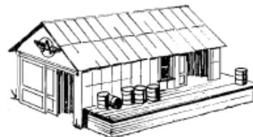
The Oil or Compound House is used to store oil, grease and other similar products in bulk amounts, also to load and deliver them to the local retail dealers. It is usually at least a small distance from the warehouse. The structure is frame with corrugated siding and roof, kept well painted and of necessity neat and clean. A truck loading dock lines one side and the building contains an inside dock and an overnight storage for a small truck.
